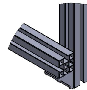
Brackets will be used to secure the profile bars on their exact position. Total of 64 such Brackets will be used.
