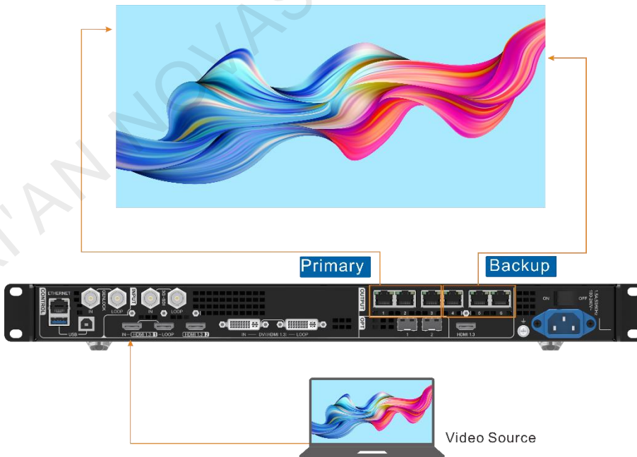
Figure 5-27 Ethernet port backup connection
