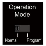
According to the silk prints nearby ("Program" for firmware update, "Normal" for RS232 transmission), change the switcher positions to set RS232 port's function.
